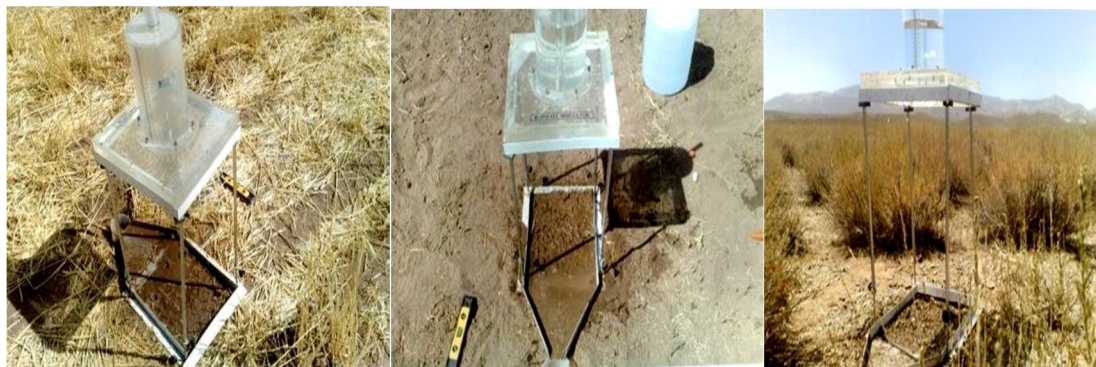
Figure 3. Proper installation of the rain simulator in rangeland, rain-fed and abandoned rain-fed land-uses
